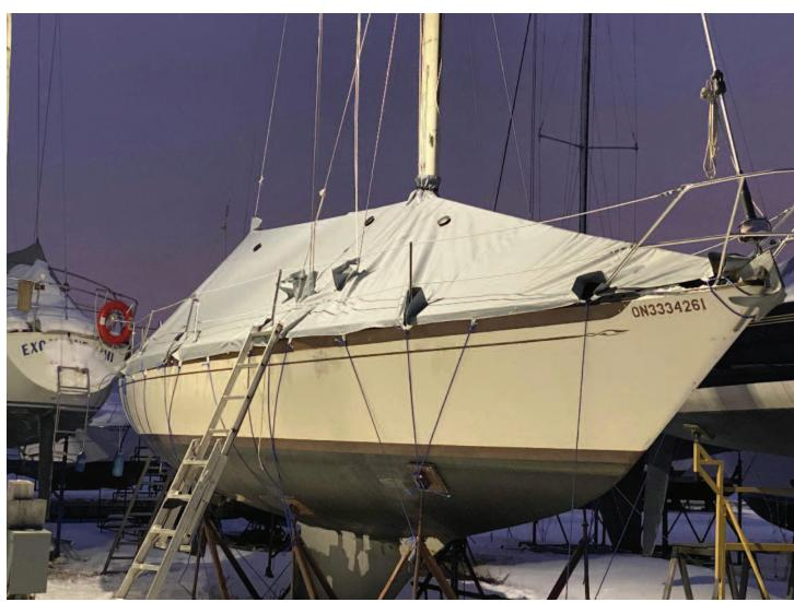
unstepped the mast, we'd be able to cover the boat more easily, but not without other issues: the hassle of stepping and unstepping the mast; the expensive of tarps big enough to cover the boat as they tend to wear out quickly; building a framework to support the tarp so that snow would slide off.
