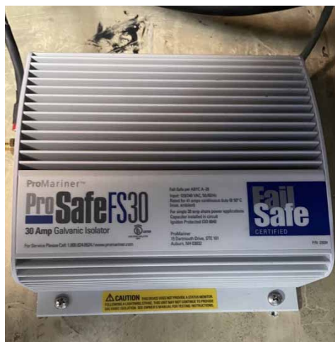
From left to right: Teak replaced with Starboard, water heater pulled out, and Kapai's new galvanic isolator
