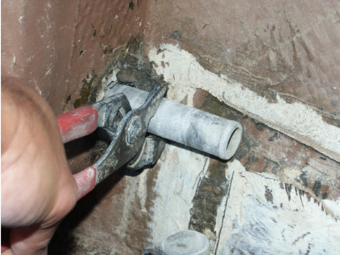
*Removing pipe. (Turn and pull pipe through hull. You may need another person at other end to tap pipe with hammer and punch to push pipe through and disengage from through-hull on opposite side.)*
