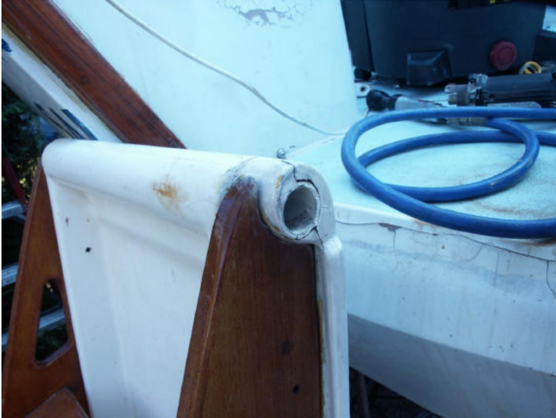
*Swim step removed (with pipe removed). Pipe slides out of swim step.*
