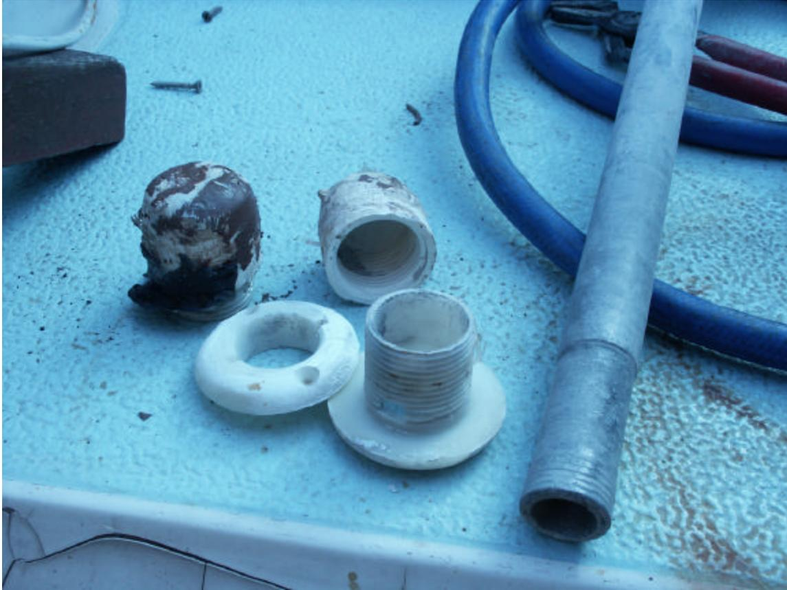
*Picture shows old pipe and plastic through-hulls and cap.*
