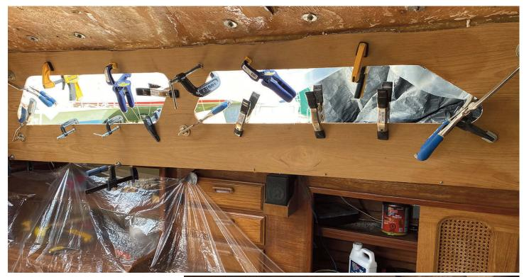
fiberglass opening onto the wood templates, then used the original plastic portlights as guides for new openings. It took a bit of futzing, but we were able to get the openings marked on both templates so that each set of portlights would be symmetrical with the other side of the cabin - or at least no glaring differences. The openings were cut out with a jigsaw and were carefully sanded to get them as smooth and straight as possible.
