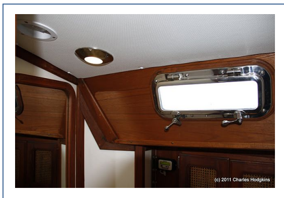
New overhead LED lights, headliner, and opening ports
