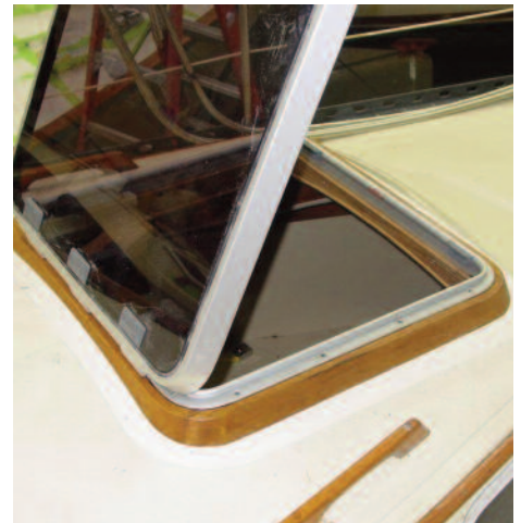
Galatea's front hatch replacement
